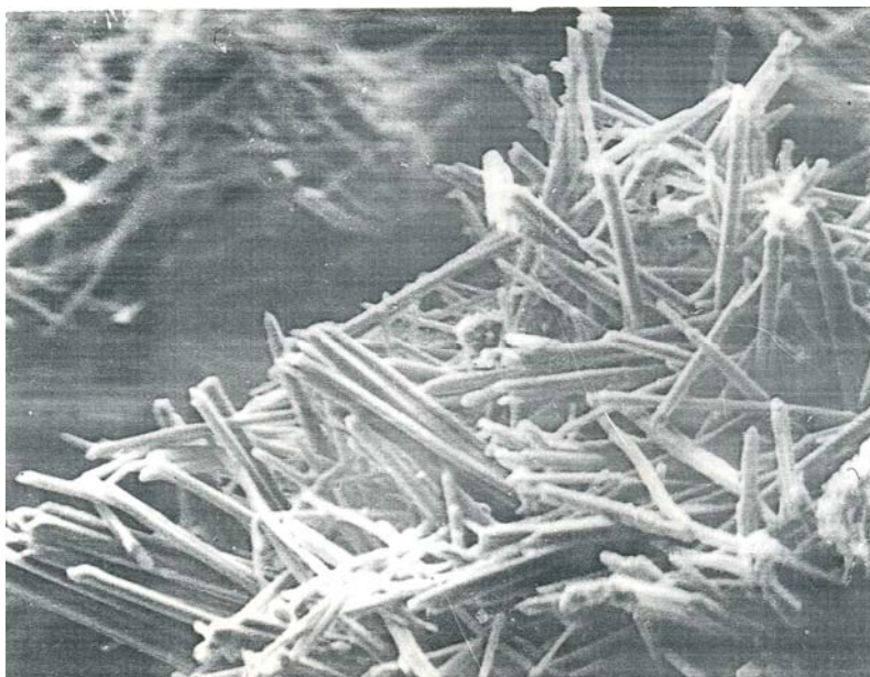
Figure. Electronic Microphotography of Ettringite Crystals 3\text{CaO}\cdot\text{Al}_2\text{O}_3\cdot3\text{CaSO}_4\cdot32\text{H}_2\text{O}
