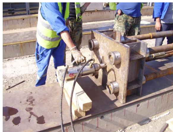
Photo 3. QYC 240 type jack in the process of calibration
