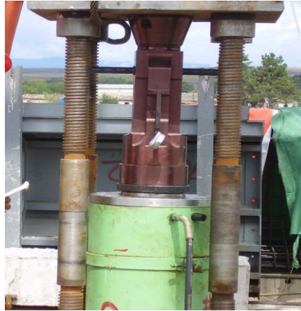
Photo 2. Dynamometre placed on YDT 3000 type jack
