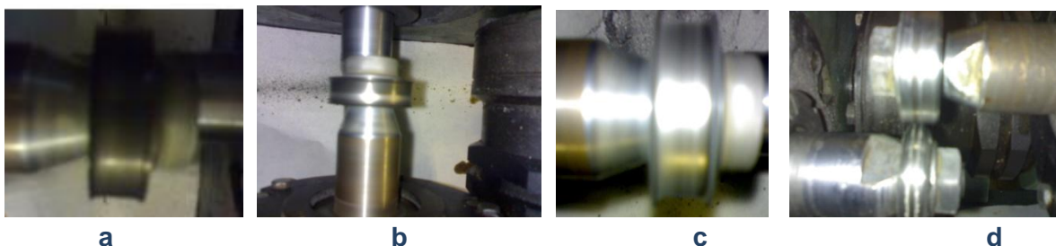
Fig. 2. The interacting surfaces with initial line and point contact of surfaces (a) the first stage of destruction of friction modifier (darkened surface), (b) surface with partial and total (c) removal of friction modifier and (d) the initial point contact of surfaces
