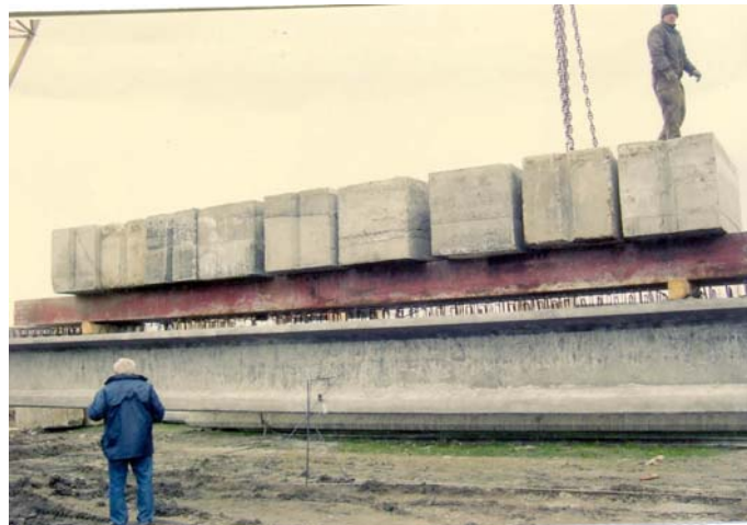
Foto 2. General view of the beam test
